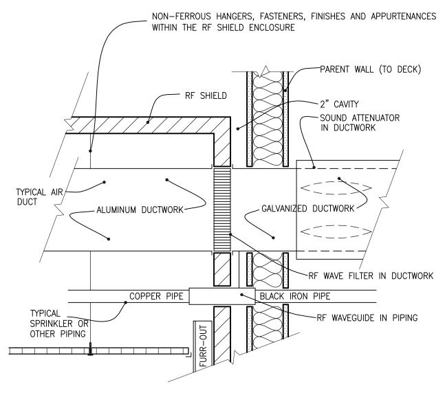
NOTE: RF WAVEGUIDES AND FILTERS FURNISHED AND INSTALLED BY RF SHIELDING SUPPLIER. DUCTWORK, PIPING, WIRING AND CONDUIT INSTALLATION MUST BE CAREFULLY COORDINATED BETWEEN CONTRACTOR'S FORCE AND THE RF SHIELD VENDOR, IN ACCORDANCE WITH THE MRI MANUFACTURER'S SITE PREPARATION REQUIREMENTS.
