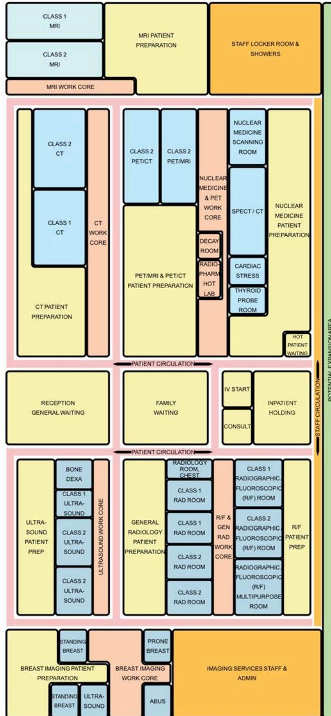
Figure 3.1: Imaging Services Departmental Functional Diagram.
