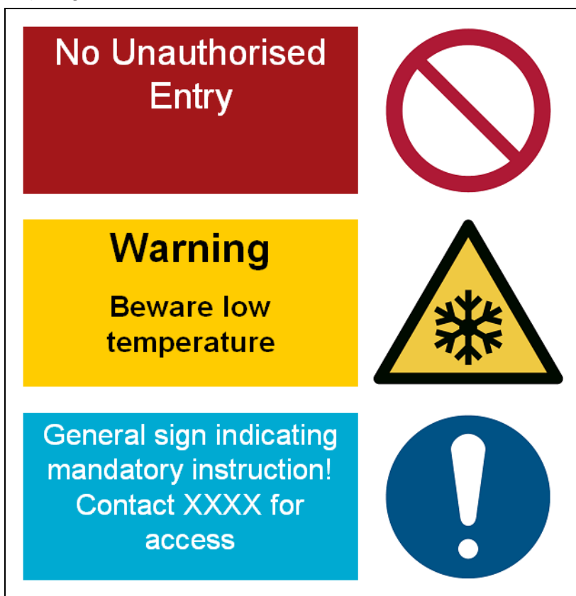
Figure 3 Cryogen Hazard sign
